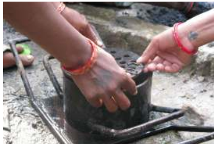
Two women from the Kapilvastu producer group working together to finalize a bio-briquette
