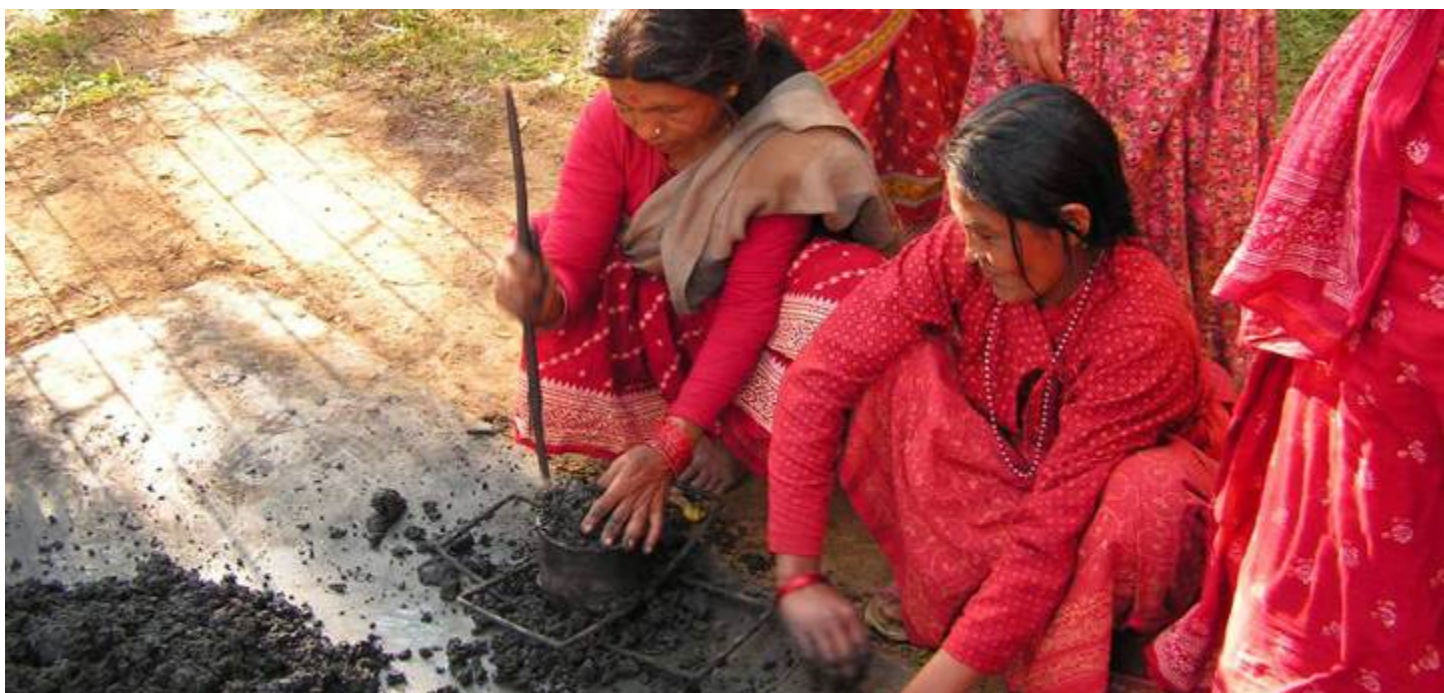
Group of women compressing a mix of charred banmara, water and soil into a briquette mould
