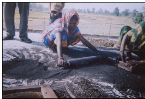
Example of grinding the charred biomass with use of a hand roller
